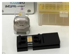
Assemble of U-type fluidic module and prism holder 1 and do experiment
