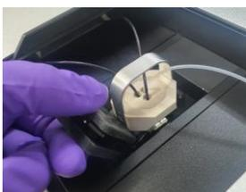
Assemble of S-type storage fluidic module and prism holder 1 and store at 2~8°C, you can perform another test using prism holder 2
