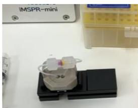
Detachment of S-type storage fluidic module and prism holder 1
